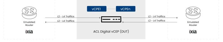
The DUT above is a COTS server with Intel Xeon E5- 2680 v2 processor. Following performance figures were measured Per Core with vCPE Fast Path optimized using Intel DPDK.
