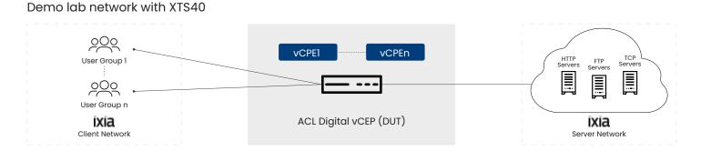
The DUT shown in the diagram above is a COTS server with Intel Xeon E5-2680 v2 processor. Following performance figures were measured Per Core with vCPE Fast Path optimized using Intel DPDK.
